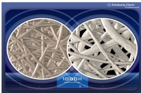
Conventional hand towels have compressed packed fibres which cause water to sit on top of the towel. This slows absorbency and can result in increased towel usage.
